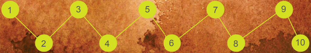
Sampling at several locations in a zig-zag pattern to ensure homogeneity.
